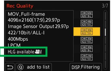
Filtering by HLG-compatible setting can be applied.
