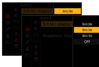
When the DMW-XLR1\* is attached, audio is down-converted to a format suitable for the connected HDMI external device before being output.
