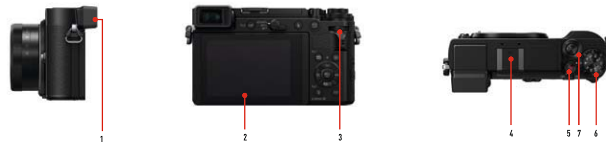
1: Tiltable LCD Viewfinder 2: Tiltable 7.5 cm LCD touchscreen 3: Thumb control dial 4: Hot shoe 5: Video record button 6: Mode dial 7: Index finger dial
