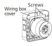
©Release the clamp, strip the power cord (where the ground wire must be 10 mm - 15 mm longer than other leads), and twist the separate copper core wires into a bundle. Then, connect the wires according to the following wiring method (make sure that the wiring screw column of the wiring terminal is pressed on the copper wire and the copper wire is not exposed). Secure the power cord with a clamp and install the wiring box cover back. (See Page 9 for the wiring diagram)
