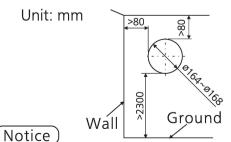
Do not drill the mounting hole in the beam, pillar, load bearing wall; otherwise, safety of the building structure may be affected. Keep the mounting hole away from electric wires in the wall, to avoid damage to the wires.
