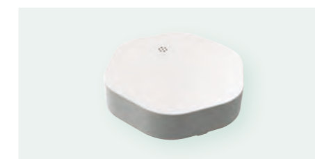
Water leakage sensor. Two sensing pads under the body activate when water is present between the two pads. Detecting the water, the sensor reports the event to the controller (and BEMS).
