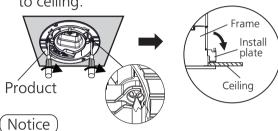
Ensure the tighten torque in the range of 60 cN·m to 120 cN·m. Product may fall off when torque not enough, may damage when torque too large.
