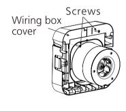
© Release the clamp, strip the power cord (where the ground wire must be 10 mm - 15 mm longer than other leads), and twist the separate copper core wires into a bundle. Then, connect the wires according to the following wiring method (make sure that the wiring screw column of the wiring terminal is pressed on the copper wire and the copper wire is not exposed). Secure the power cord with a clamp and install the wiring box cover back. (See Page 9 for the wiring diagram)
