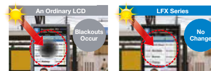
Direct sunlight raises the LCD panel temperature and causes blackouts.
