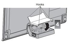
Ensure that the TV does not hang over the edge of the base.
