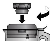
4. Align the "▽" icon on the bottom of the blender jug with the "△" icon on the body, then place blender jug onto the base.
