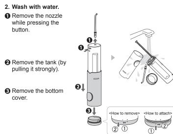
The tank and the bottom cover can be washed in a dish washer.
