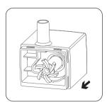
3. Remove the impeller.
