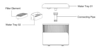
2 Put the cleaned filter element into the filter element box. (Replacing the filter element: remove the water tray 02 and replace the filter element.)
