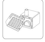
2. Remove panel with holding the top cover.
