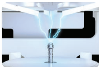
2 Electrical discharge is applied to the water.
