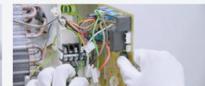
Pull out main PCB, screw-free design makes it easy to remove PCB.
