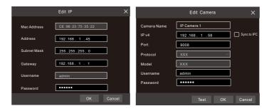
④ Click ■ to edit an IP camera as shown on the above left. Enter the new IP address, subnet mask, gateway, username and password of the camera. Click "OK" to save the settings.
