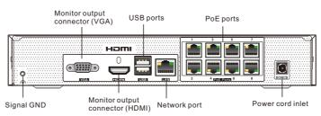
Signal GND: Connect this terminal with the Signal GND terminals of the devices in the system for signal ground. When oper- ating the recorder and the devices in the system without signal ground, oscillation or noise may be produced.
