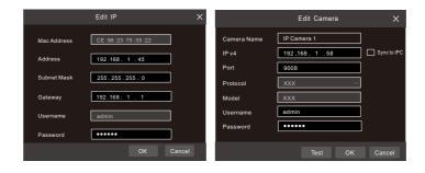
④ Click ■ to edit an IP camera as shown on the above left. Enter the new IP address, subnet mask, gateway, username and password of the camera. Click "OK" to save the settings.
