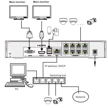
Max. 8 cameras can be accessed to the NVR (either via PoE ports or network)
