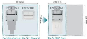
Combinations of KV-SL1066 and Flatbed option (KV-SS081) → Large space is required: 750 mm x 800 mm
