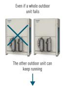
Even if a compressor in a single system fails The other compresso can keep running
