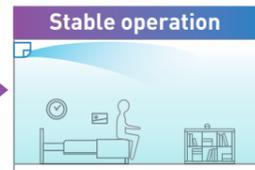
When the room reaches the set temperature, the airflow automatically switches to ceiling airflow so that cold air doesn't hit the body directly and occupants don't get too cold even when the air conditioner is operated for a long time.
