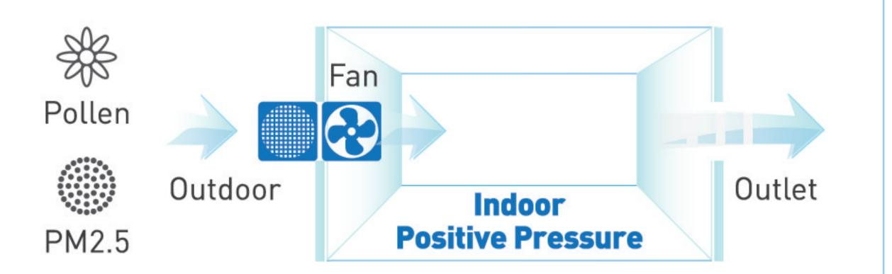
Using a supply fan, fresh outdoor air is drawn from a known location and delivered to the interior living space. The known location should be selected to ensure that the air brought in is good quality. The intake air should be purified before distribution within the living space to minimize the impact of outdoor pollutants on residents.
