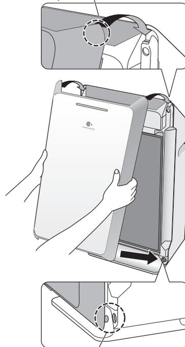
Push in the protrusion into the holes (2 places) of product and press properly.
