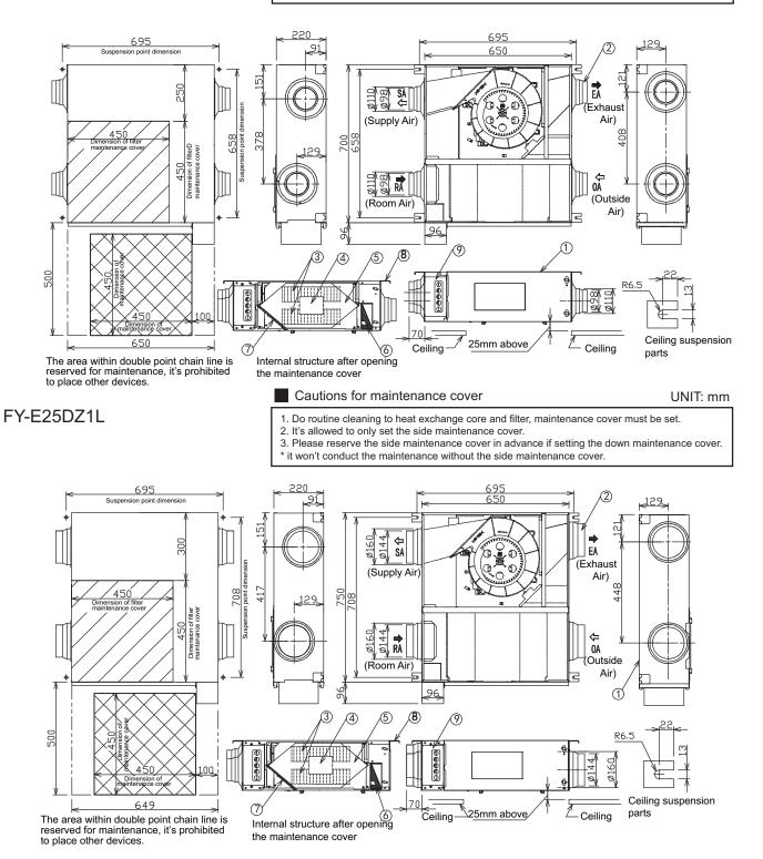
No. Part name Quantity Material No. Part name Quantity Material Frame 6 Outdoor filter 1 Galvanized steel sheet 1 1 Nonwoven fabric 2 Adapter 4 ABS 7 Indoor filter 1 3 2 PP Ceiling suspension part 4 Impeller 8 Galvanized steel sheet 4 Fan motor 1 9 Switch box 1 Galvanized steel sheet 5 Heat exchange core 1 Special paper+resin
