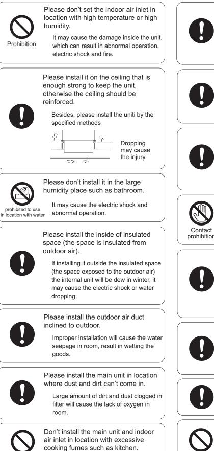
It must use the specified part during the installation (include the accessories)
