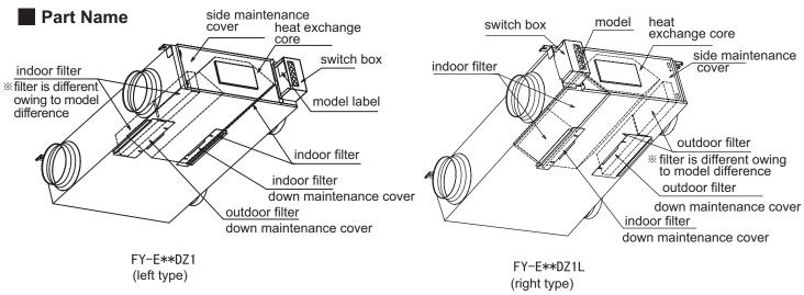
% 1 The amount of indoor filter is different owing to model difference.
