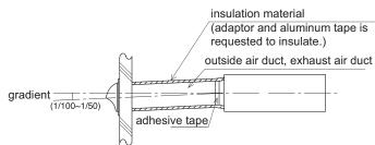
Conduct the insulation to outside of two ducts connected with outdoor (suggested material :glass wool ,thickness 25mm)
