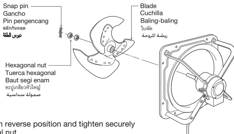
3. Mount the blade in reverse position and tighten securely with the hexagonal nut.
