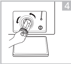
4 Open the filter by turning to the counter clockwise
