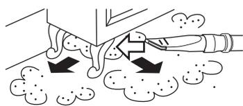
For locations where the 2-Step Nozzle will not enter, connect the Hose to the Blower and blow the dust out.
