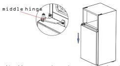
11. Take out the top hinge and top hinge cover from the accessory bag in the refrigerator. Put down the freezer door on middle hinge vertically, then install the top hinge and hinge cover, finally to install the cover plate you previously removed
