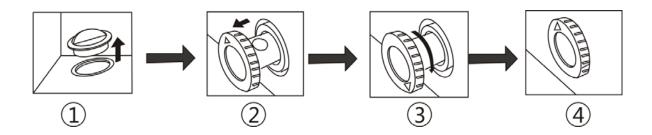
1. There is a water conduit at the bottom of the freezer, when defrosting, extract the rubber cover, defrosted water will drip into the hole and flow out.
