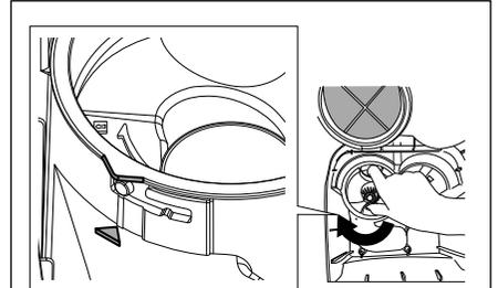
Align the arrow to pull out the Pre-Filter.
