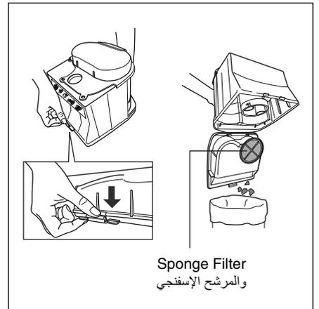
③ Removing and cleaning the Pre-Filter.
