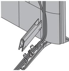
Using the cable clampers (supplied), arrange the cable.
