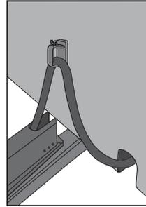
4 Arrange left and right side of the cable dressing as shown below:
