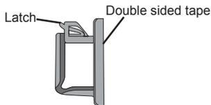
2 Open the latch and arrange the cable to clampers.
