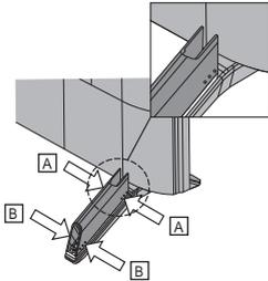
2 Fix the cable dressing to pedestal and then close the pedestal cover. Please ensure the pedestal cover fully fix.
